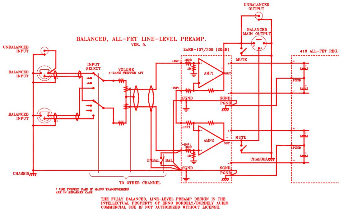
Fig. 4. Two EB-107/309 amps wired for balanced operation, using 4-gang stepped attenuator
